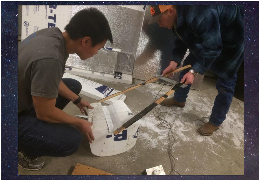
Figure 2: Cutting Cross-Section with Hot Wire
