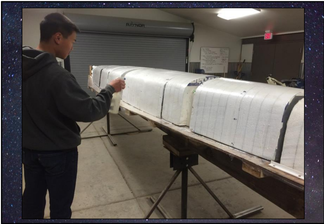
Figure 8: Applying Form Oil to Mold
