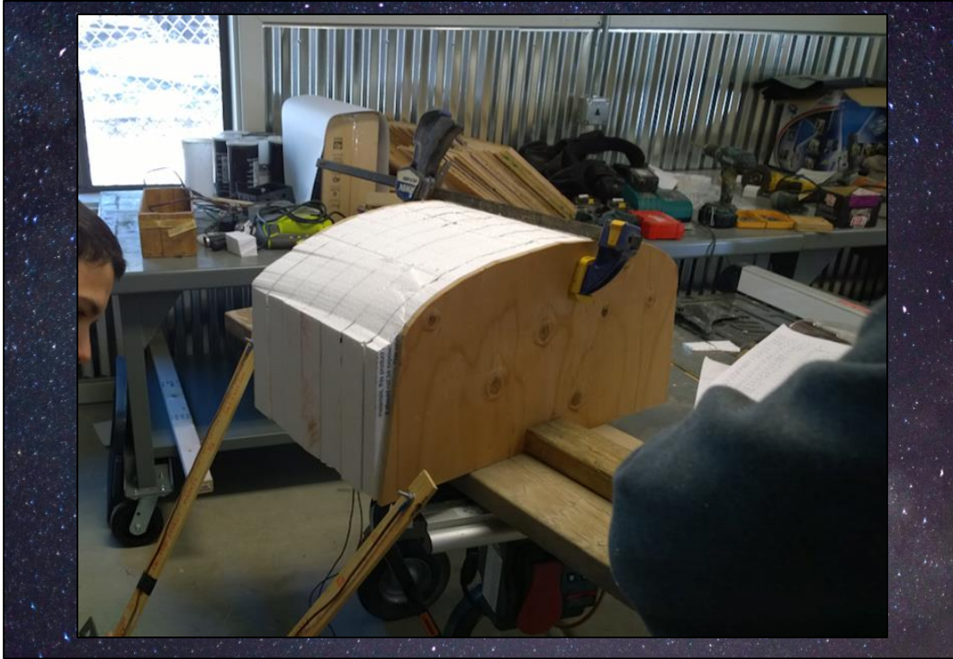
Figure 1: Cutting Cross-Section with Hot Wire
