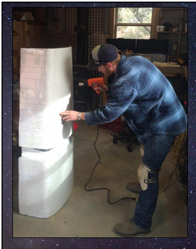
Figure 6: Applying Shrink-wrap to Mold Section
