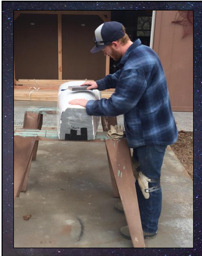
Figure 5: Placing Joint Compound on Mold
