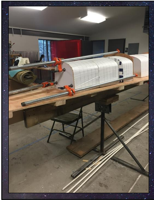
Figure 3: Gluing Sections Together
