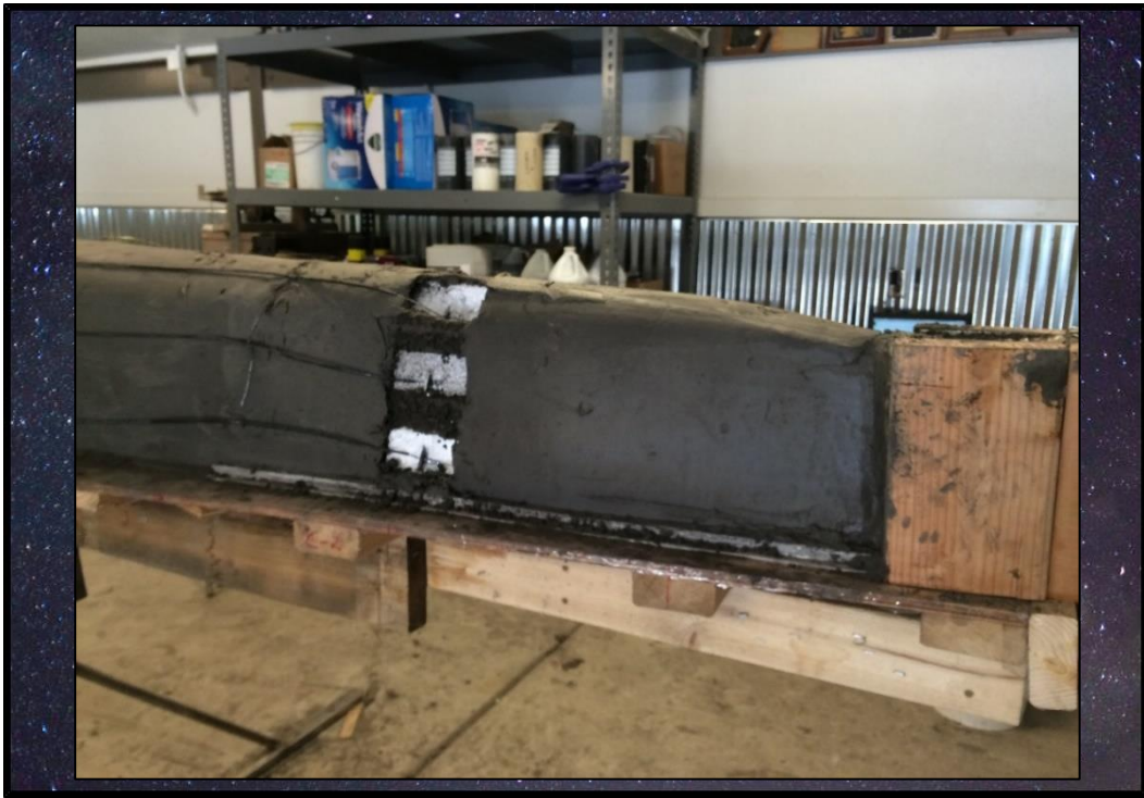
Figure 11: Post-Tensioning Placement on Bow Bulkhead
